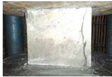
Concrete cube specimens testing for compressive strength
