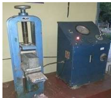
Concrete specimens testing for flexural strength
